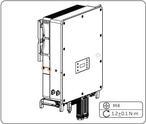
Figure 26-13 Lock the screws
